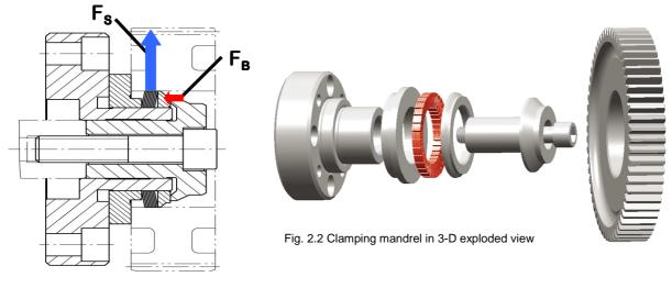
Fig. 2.1 Clamping mandrel with bonded disc pack
