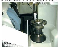
Fig. 15.2 Clamping mendrel used to grind automotive spur gears
