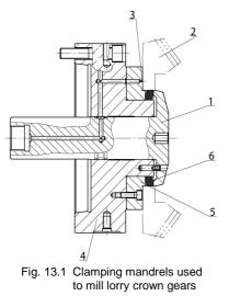
The bonded disc pack clamping mandrel is loaded by an automatic component load unit. The mushroom bushing (1) has a large insertion groove to prevent collisions. Loading is
