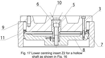
The hollow shaft (1) has pre-drilled mounting bores at each end with diameters of 195.0 mm and 384.5 mm, respectively and adjacent flat surfaces (see Fig. 16). Flat-mandrel centring inserts Z1 and Z2 with large insertion grooves are inserted into these mounting bores and then clamped by hand by turning the hexagon socket head cap screws (4 and 5).
