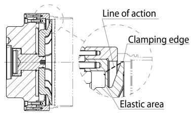
clamping elements Diaphragm with diameters of up to 1200 mm have been developed and manufactured especially for large rotors in aircraft engines in many cases. These elements work according to the same principles as the clamping elements described before. Clamping is also effected by a shift in the line of action (see Fig. 9, detail view). The fulcrum of the inner end of the line of action is located in the elastic area of the diaphragm. The clamping element is slotted from the inner edge only.
