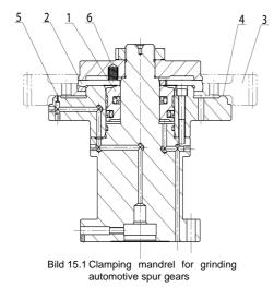
This clamping mandrel has a flat-mandrel clamping element (see Chapter 2.3.) The clamping surface of the spur gear is very short. The element is actuated hydraulically from the machine spindle. The piston (1) is pressed against the clamping element (2) of the flat mandrel, thereby actuating it. In the process, the spur gear (3). The air-system control unit (5) monitors the correct seating of the spur gear. The clamping system
