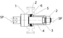
Fig. 12 Clamping mandrel for gear noise testing
